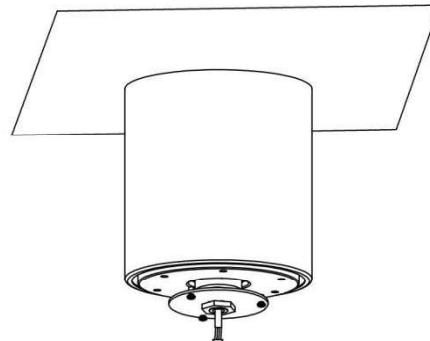
Ensure all wires are tucked neatly into the motor casing to avoid any damage.
