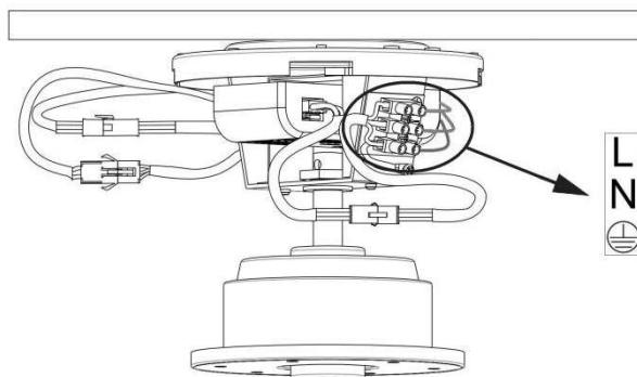
Fix the Earth cable and complete all electrical connections at the mounting bracket.
