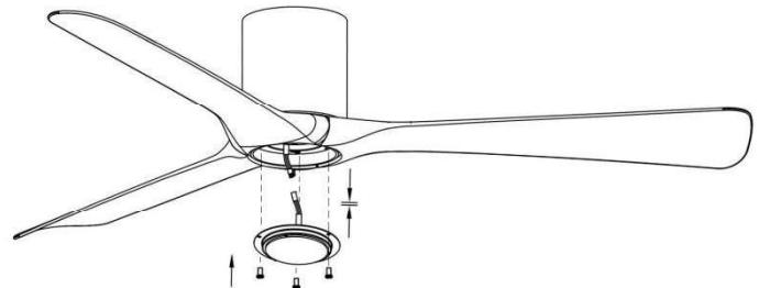
Connect LED lights with motor using by quick plugs.
